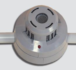
Made of ABS, equipped with bayonet contacts that allow detectors to be replaced without disconnecting their cables. They are manufactured in a standard 22mm version, which allows the tubes to enter when the installation is visible, and 10mm with an internal entry for recessed installations.
